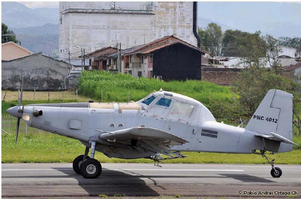
**Figure 2.8.** Photograph of AT-802 Spray Plane<sup>225</sup>
