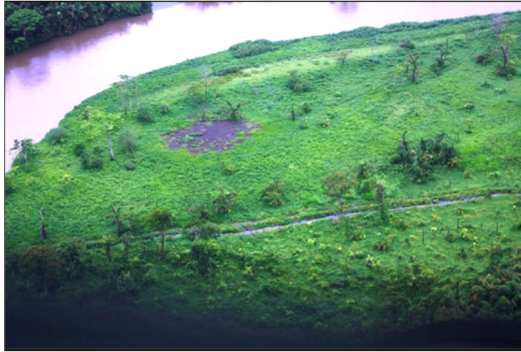
Figure I.39. Photograph taken on 15 June 2011 showing reduced flow and channel widths in the ‘Caño’, vegetation recolonising the outer channel and berms, and patches of vegetation growing on the area raised by the pumping of dredge spoil.
