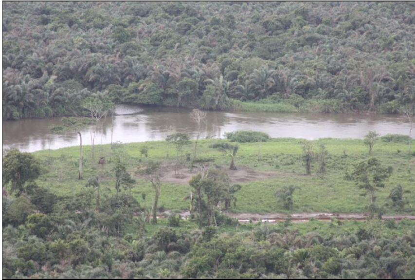
Figure I.31. Photograph taken on 29 January 2011. Discharge in the Río San Juan has decreased and flow in the ‘Caño’ has receded into the narrow, inner channel. Widening of both the outer and inner channels due to erosion and destruction of vegetation during the flood event of December 2010 can be identified. The encampment on the raised area of dredge spoil appears to have been abandoned.
