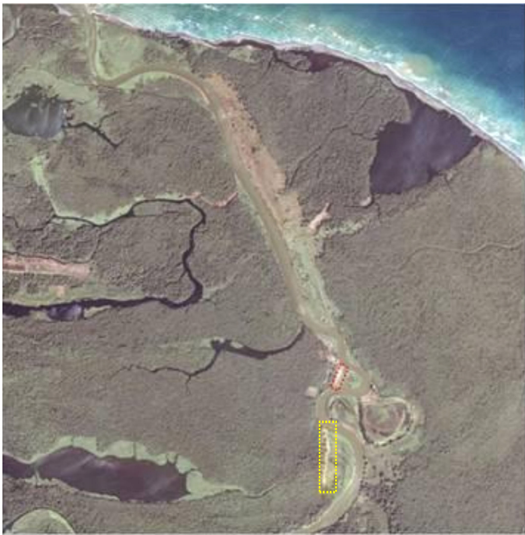
Figure Notes: Red rectangle indicates location of dredger and extended meander cut-off channel, now nearing completion. Yellow rectangle highlights a corridor that appears to have been cleared of vegetation along a tributary probably draining from Laguna la Barca at the inside of a long radius meander bend in the Río San Juan.
