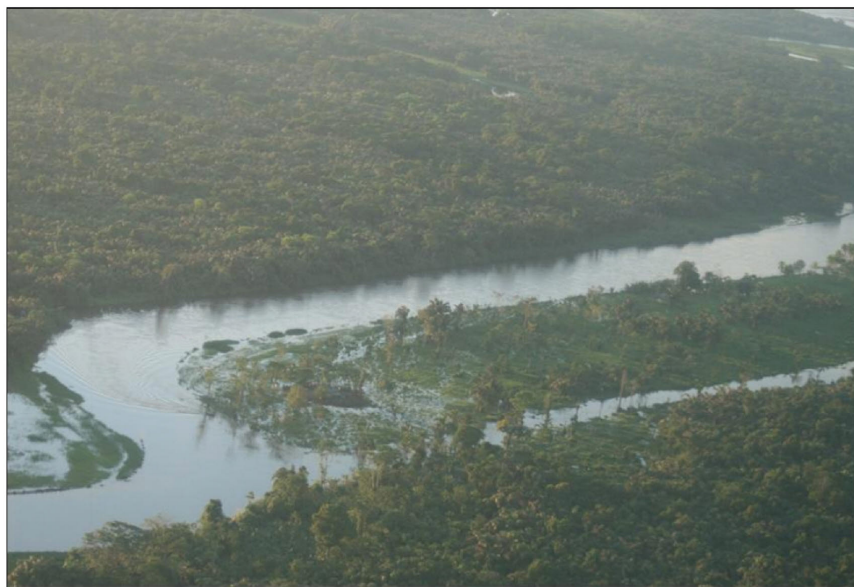
Figure I.30. Photograph of sediment-laden flood flow taken on 5 December 2010. Note high water level in Río San Juan, increased width of flow in the ‘Caño’, and water-logged area around encampment on artificially-raised ground created in late-October by dumping of dredge spoil.
