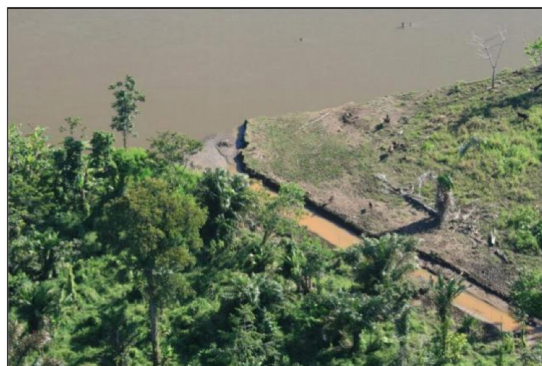
(b) upper reach of 'Caño' showing that flow is blocked from entering the 'Caño' by sand (grey sediment) deposited in its funnel-shaped mouth though silty (brown) water is still present in the channel proper
