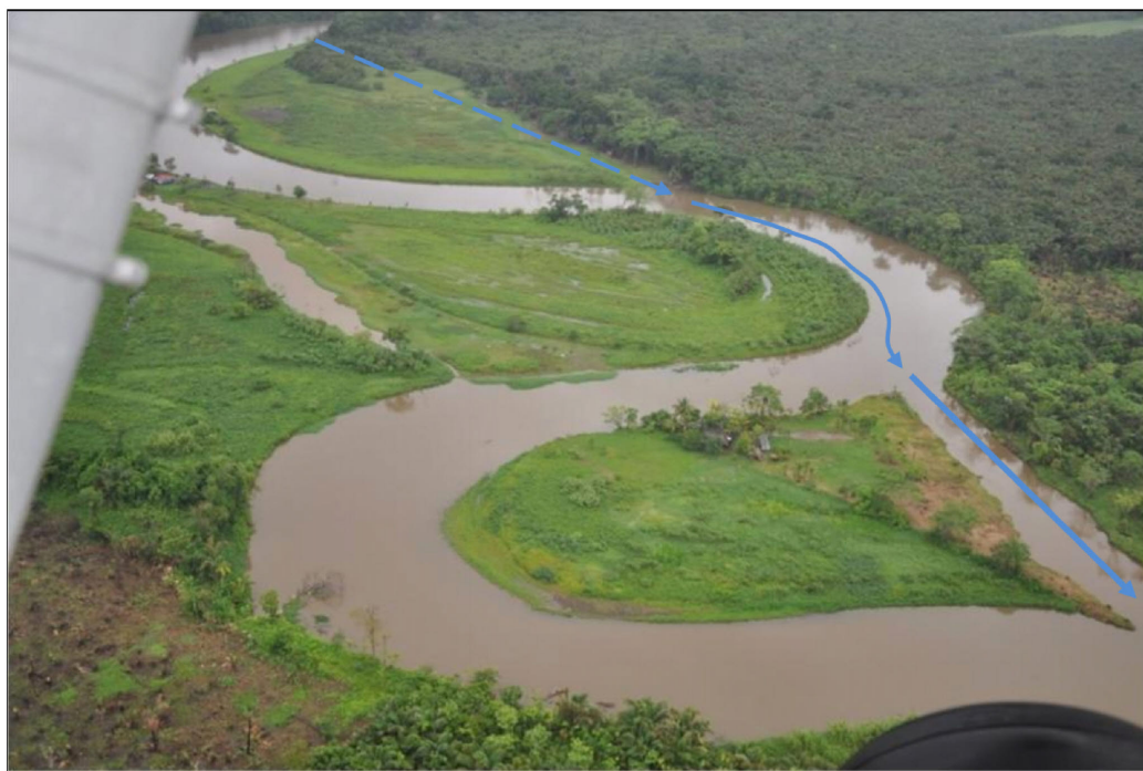
Figure Note: Arrows indicate preferred flow path if a cut-off channel were to be constructed along the line of the strip cleared of vegetation at the second bend.
