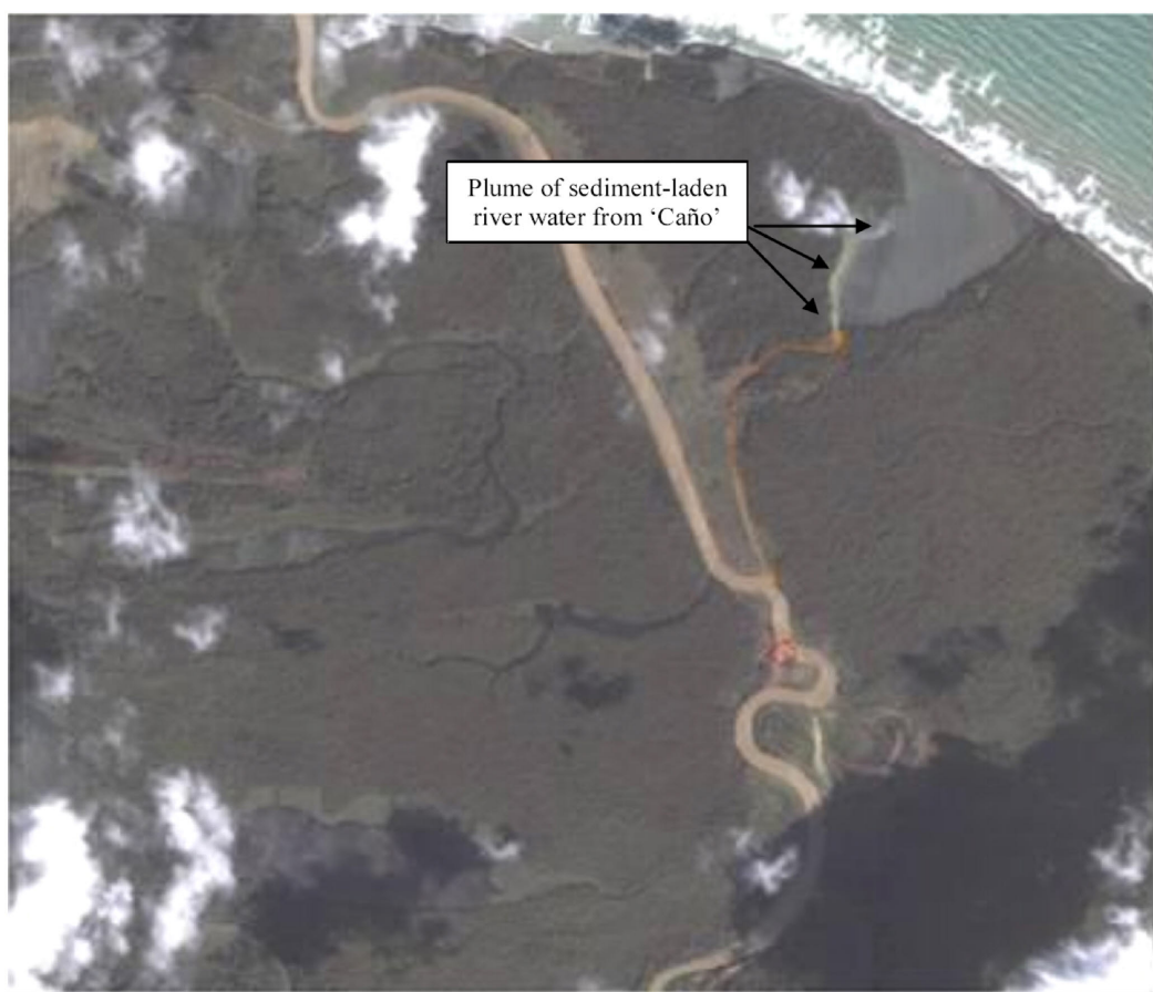
Figure Notes: Brown line indicates line of recently completed, artificially-dug channel of the 'Caño' linking Río San Juan to the Harbor Head Lagoon. Red circle indicates location of what appears to be a dredger in the artificial meander cut-off channel that is under construction.
