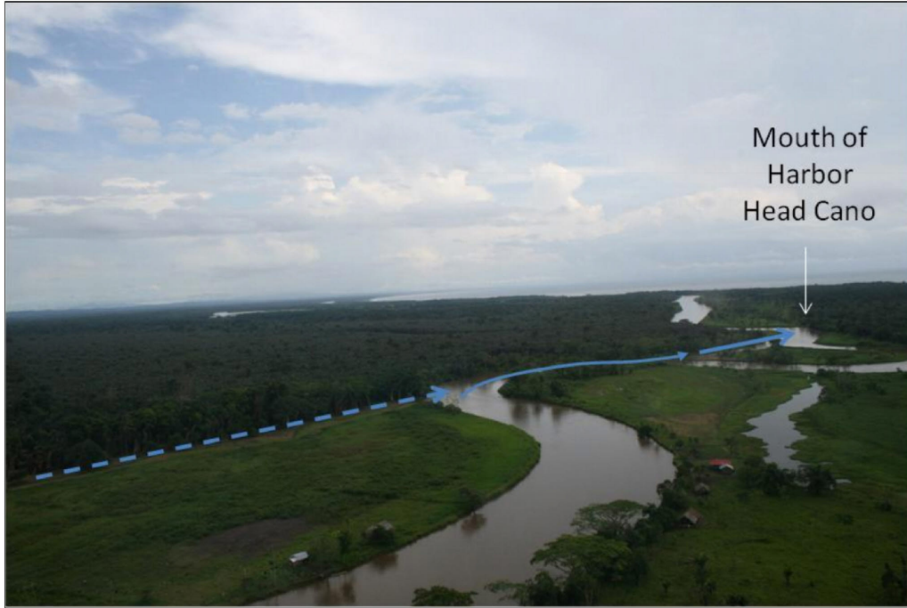
Figure Notes: Arrows indicate preferred flow path if a cut-off channel were to be constructed along the line of the strip cleared of vegetation at the second bend. The effect would be to align the flow in the Río San Juan with the mouth and heading of the 'Caño'.
