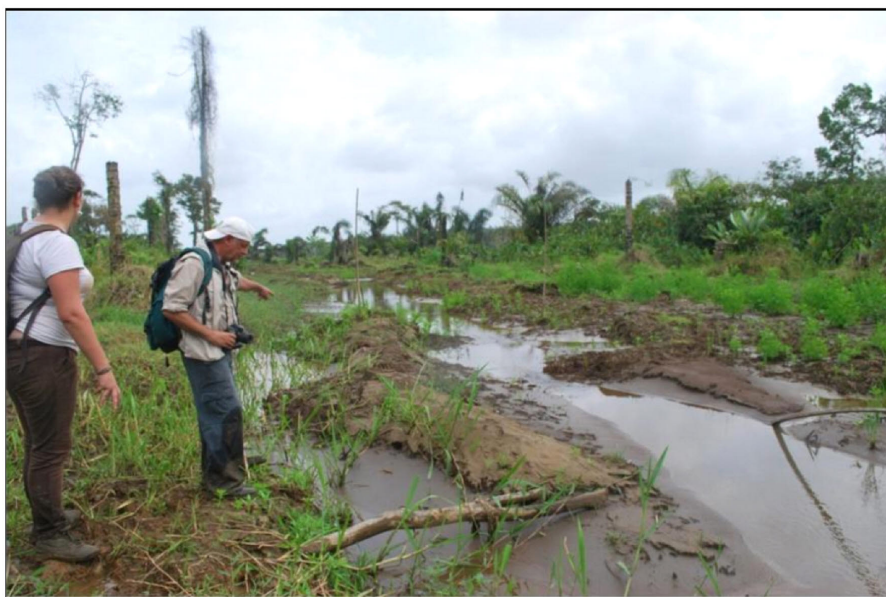
Figure I.34. Field survey of ‘Caño’ dimensions in progress at Point 2. Note heavily-silted condition of channel and its recolonisation by vegetation. Photograph taken on 5 April 2011.
