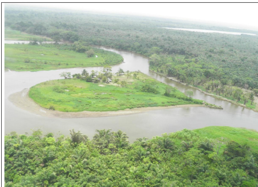
Figure 13a. Photograph of 6 April showing the cutoff of a meander to channel the flow of water from the San Juan river to the artificial canal.
