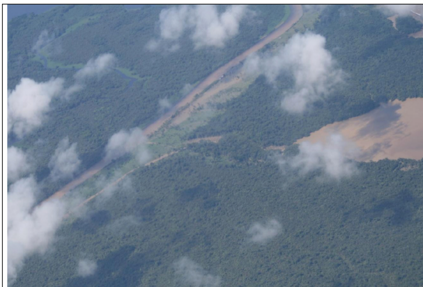
Figure 9.b. Aerial photograph of 5 December 2010 during a flood period of the San Juan river, which shows it transporting a substantial amount of sediments, and how the artificial canal opened up by the Nicaraguans allows a direct hydraulic connection between the river and the Los Portillos lagoon, which is how the sediments of the river pass via the canal towards the lagoon, altering its environmental quality.
