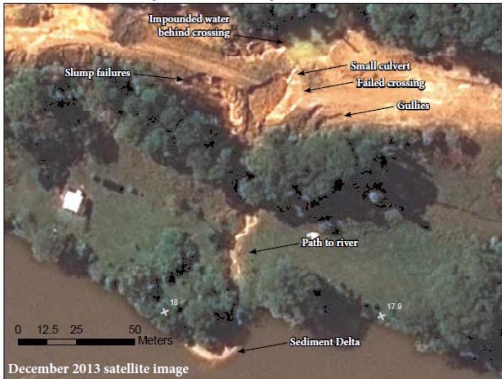
Figure 11. Eroding Site 9.4, 18 km downstream of Mojon II. High-resolution satellite image of December 2013.
