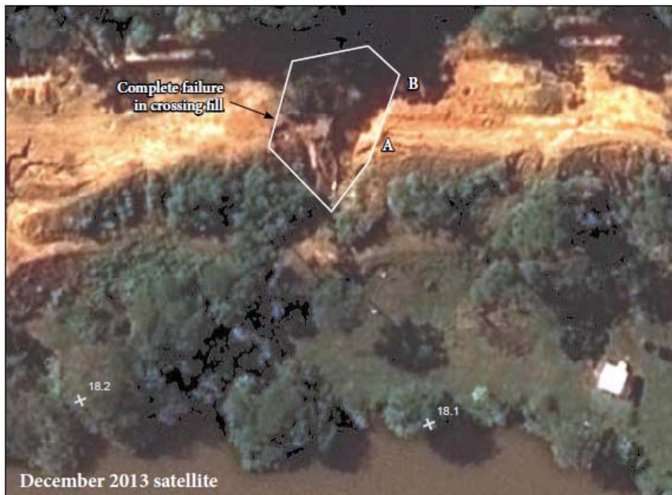
Figure 14. Eroding Site 9.5, 18.1 km downstream of Mojon II. High-resolution satellite image of December 2013.
