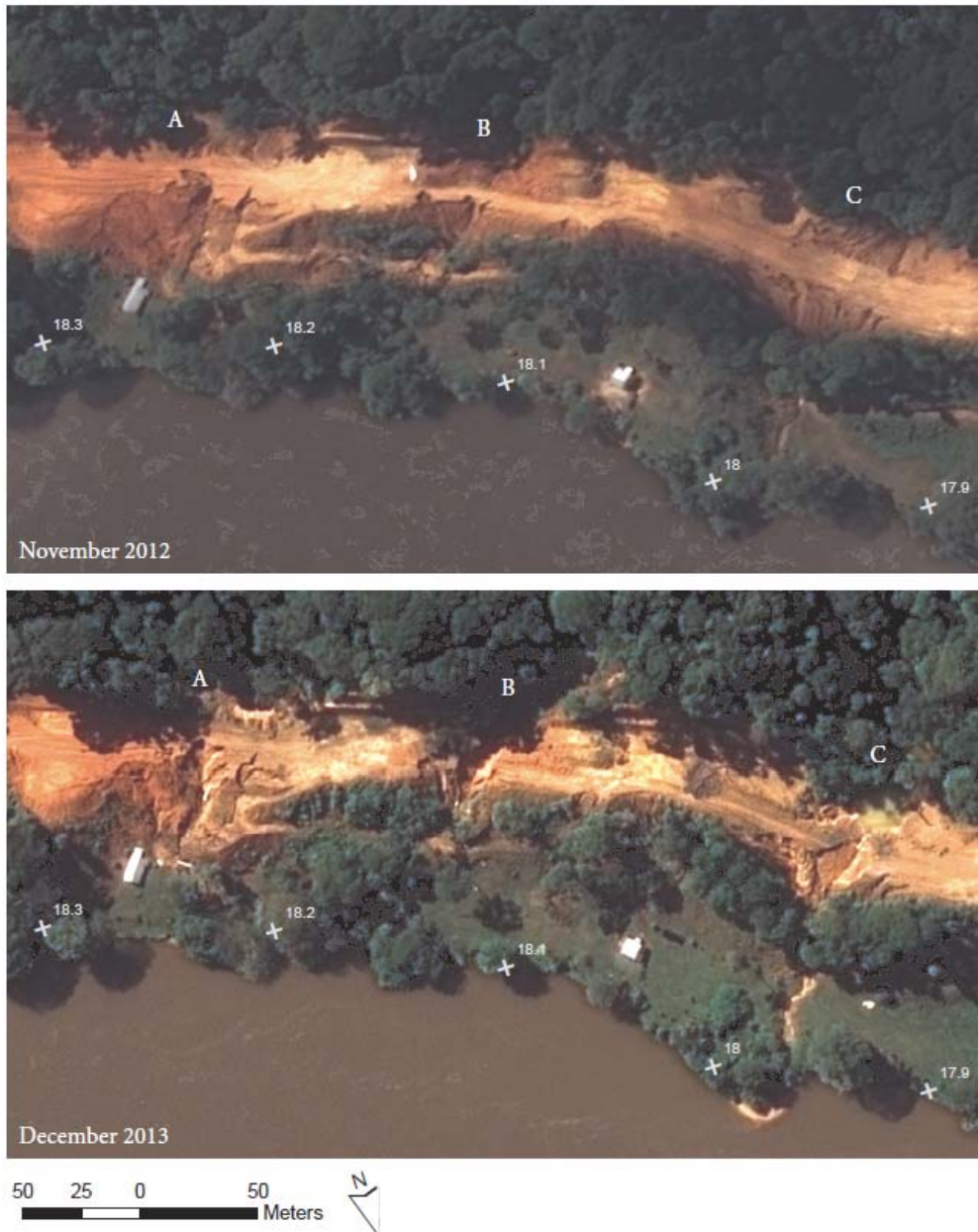
Figure 9. Progression of erosion at Las Crucitas, 17.9 to 18.3 km downstream of Mojon II. (a) Satellite image of November 2012 shows erosion has already begun on fillslopes and stream crossing fill prisms since construction. (b) Satellite image of December 2013 shows significant progression of erosion, with expansion of a gully complex at the stream crossing fill prism “A”, and washouts of stream crossings “B” and “C”.
