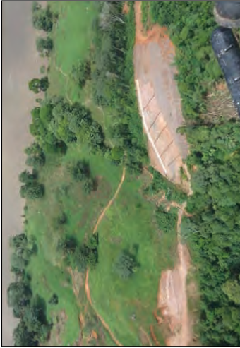
Photo 2. Aerial view of gully through pioneered but incomplete road cut (from Mende & Astorga 2013, p38).
