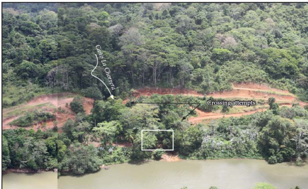
Figure 4. Oblique aerial view of Caño La Chorrera, showing multiple attempts to cross the stream, 23.9 km downstream of Mojon II border marker. White box shows location of the embayment off the main Río San Juan that was formerly a pool under a canopy of trees (as shown in Figure 5a but which is now filled for most recent attempted stream crossing for Rte 1856 (Figure 5b). Photo date: May 2, 2014.
