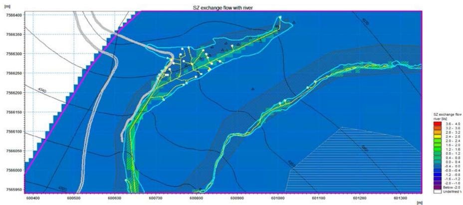
Figure 36 Simulated groundwater flow to the canal and drainage network in Northern wetland.
