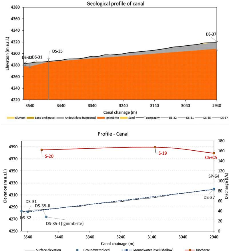
Figure 7 Geological profile C along the canal from the confluence to the border based on borehole logs (top) and profile showing spot flows and groundwater levels (bottom).
