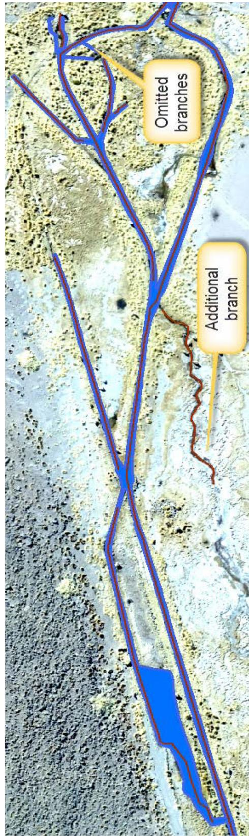
Figure 12 Artificial channel alignment in the upstream end of the Southern Catchment. The red lines represent the hydraulic model, the blue polygon is the shape file from DIREMAR showing were the canals/conveyors are located.
