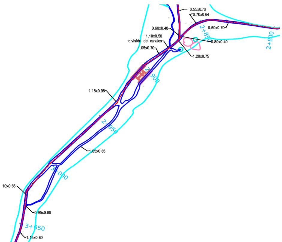
Figure 21 A close-up of the information of width and depth for canals in the Main Canal from chainage 2800 meters to chainage 3100 meters (no measurements from chainage 2450 to chainage 2800.)
