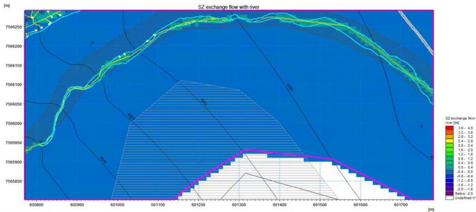
Figure 39     Groundwater discharge to the canal along the Zone 4 ravine section
