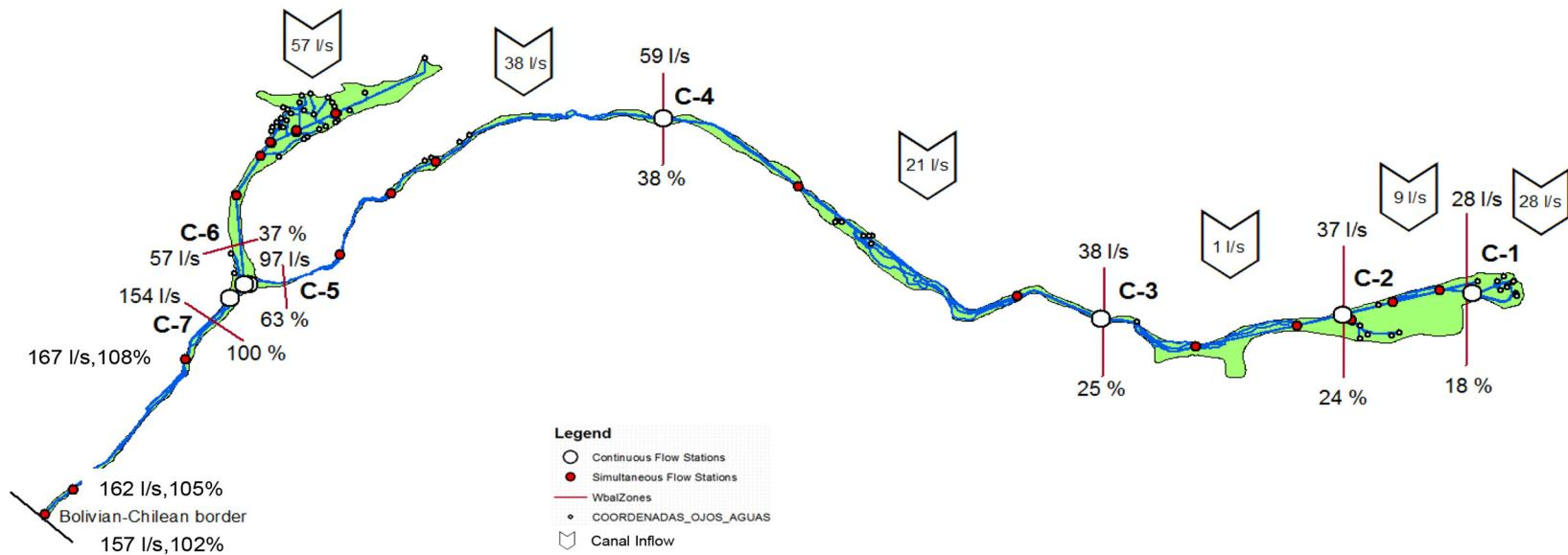
Figure 34 Mapping of flows and net inflows based on simultaneous mean canal flow measurements (in l/s), Annex C.
