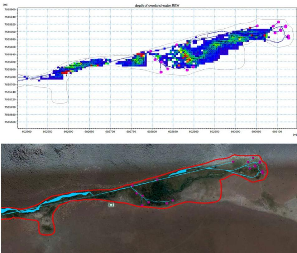
Figure 31      Simulated water depth and flow in the Southern Wetland
