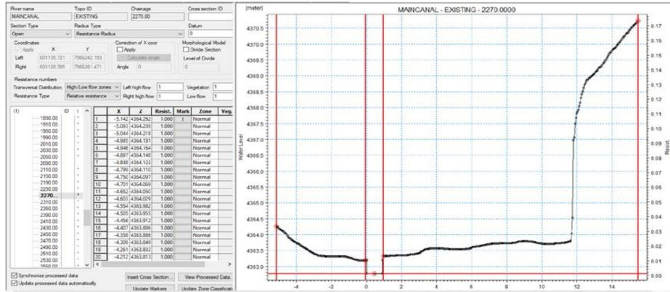
Figure 28 Canal cross sections organised in the MIKE11 cross section database.
