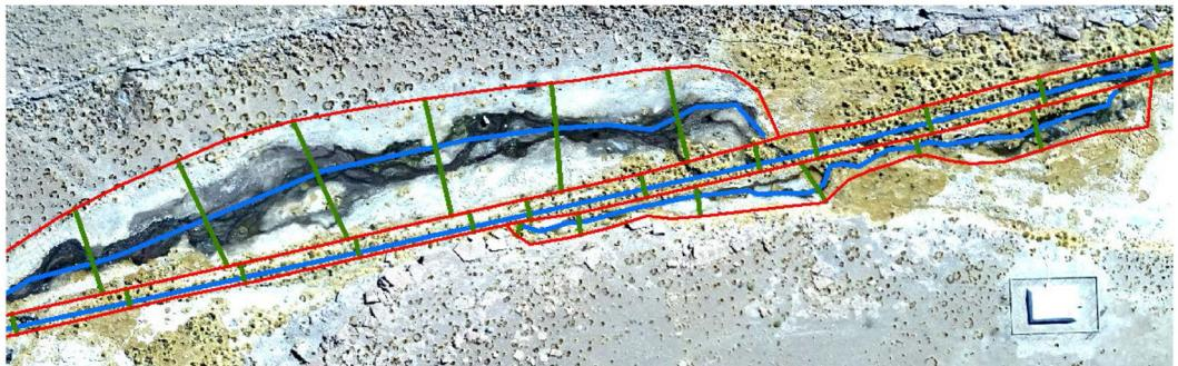
Figure 26 Example of how to define the extent of each canal by using alignment lines (in red). Blue lines represent canals and the green one the cross sections in the canals.
