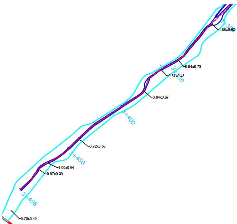
Figure 23 A close-up of the information of width and depth for canals in the Main Canal System from approximately chainage 3300 meters to the border.
