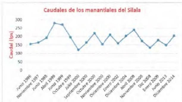
Figure 5.4. Total estimated flow of the Silala springs, taken from SERGEOTECMIN report (2002)
