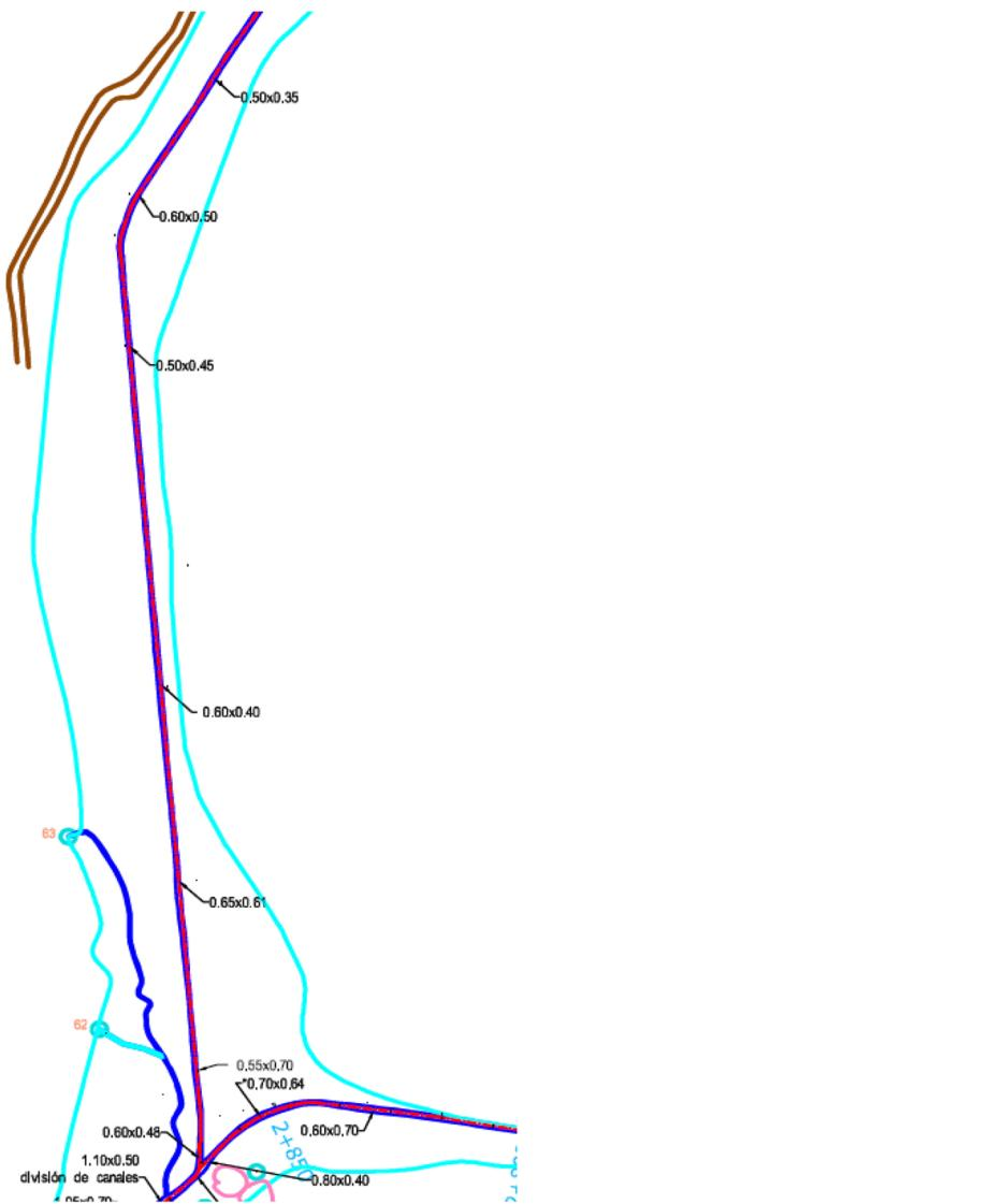
Figure 25      A close-up of the information of width and depth for canals in the Northern Canal.
