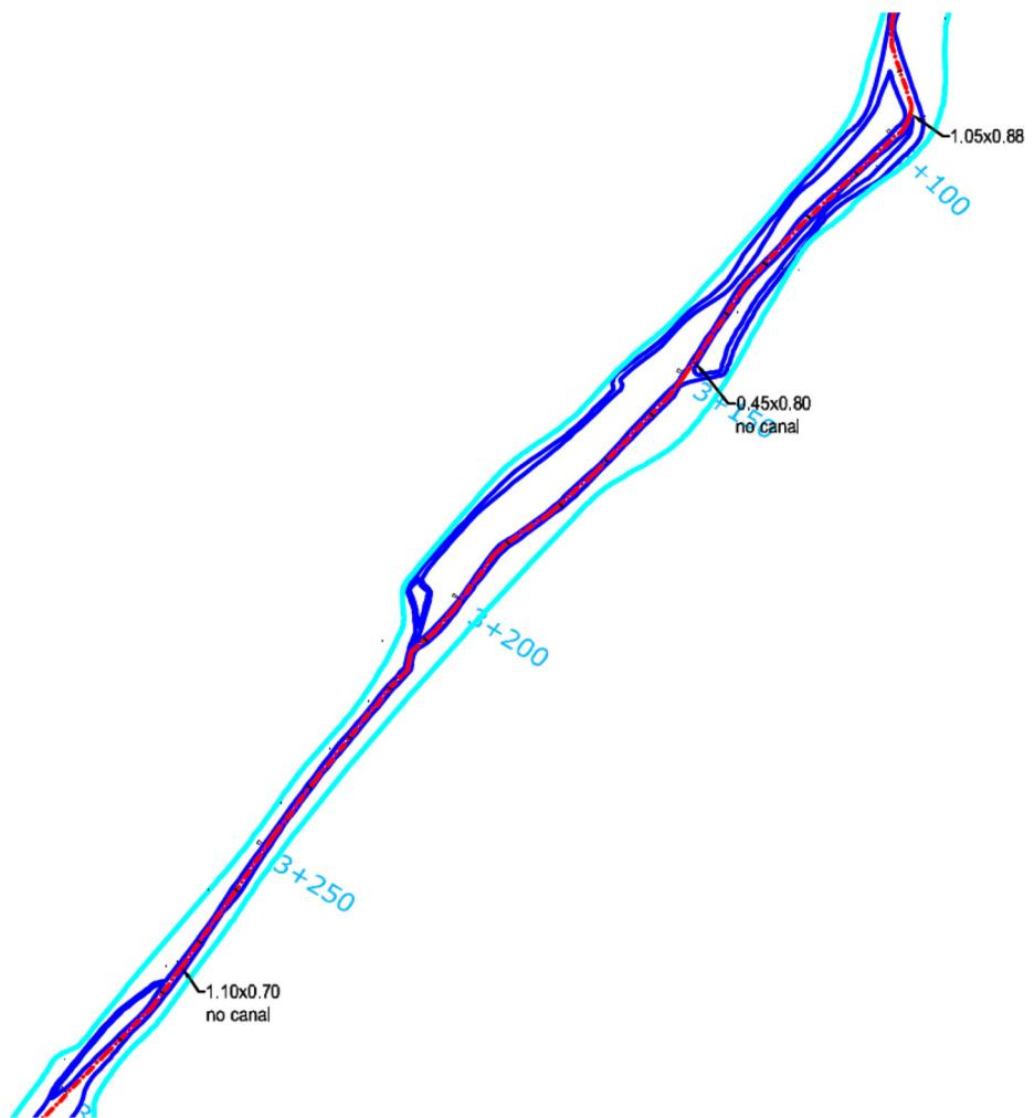
Figure 22 A close-up of the information of width and depth for canals in the Main Canal from chainage 3100 meters to chainage 3300 meters.
