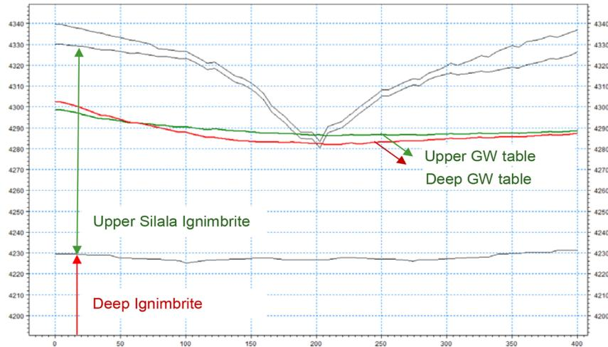
Figure 40 Cross section at the border showing groundwater layers and simulated groundwater table
