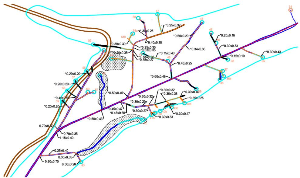
Figure 24 A close-up of the information of width and depth for canals in the Northern Canal.
