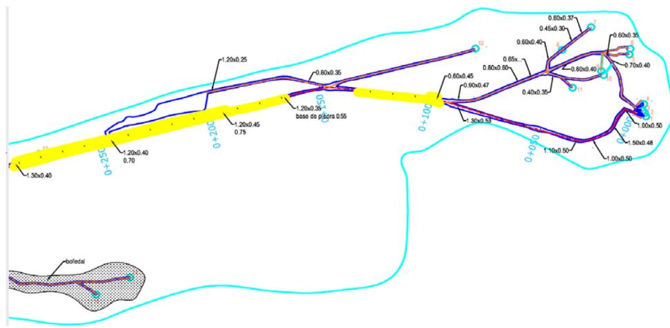
Figure 14 A close-up of the information of width and depth for canals in the Main Canal System from upstream end to approximately 300 meters downstream (Southern wetland).
