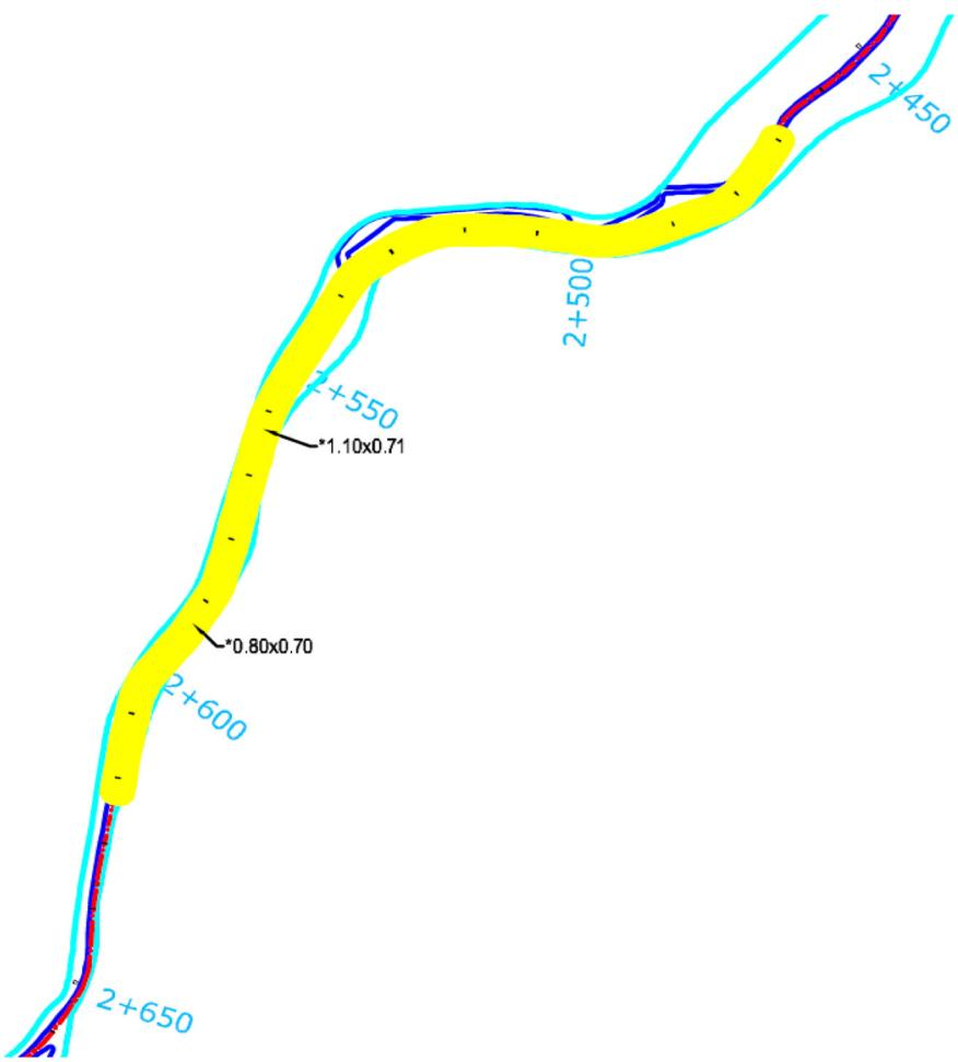
Figure 20 A close-up of the information of width and depth for canals in the Main Canal System (southern) from chainage 2450 meters to chainage 2650 meters (no measurements from chainage 2000 to chainage 2450).
