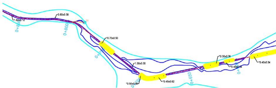
Figure 16 A close-up of the information of width and depth for canals in the Main Canal System (southern) from chainage 600 meters to chainage 900 meters.
