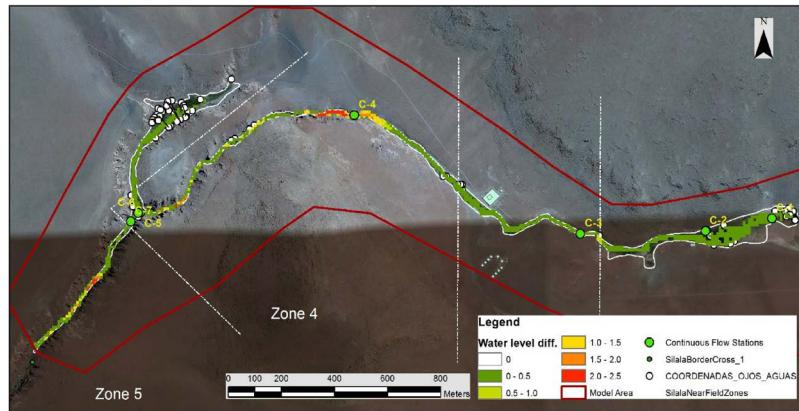
Figure 2 Change in overland water depth between the 'Baseline' and the 'No Canal' scenario.
