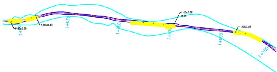
Figure 19 A close-up of the information of width and depth for canals in the Main Canal System (southern) from chainage 1500 meters to chainage 2000 meters.
