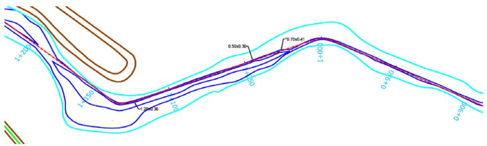
Figure 17 A close-up of the information of width and depth for canals in the Main Canal System (southern) from chainage 900 meters to chainage 1200 meters.
