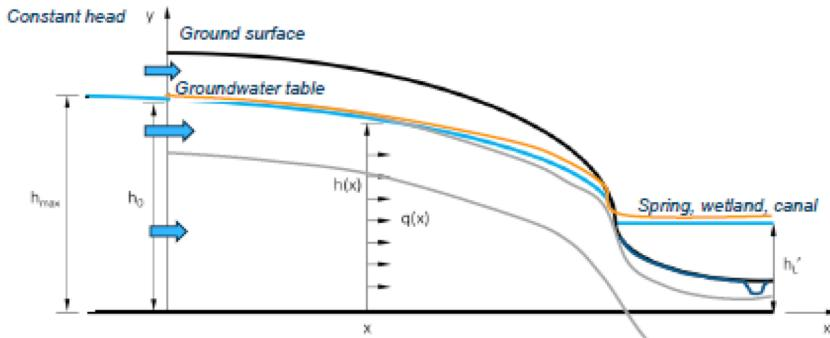
Figure 4 Illustration of groundwater boundary condition
