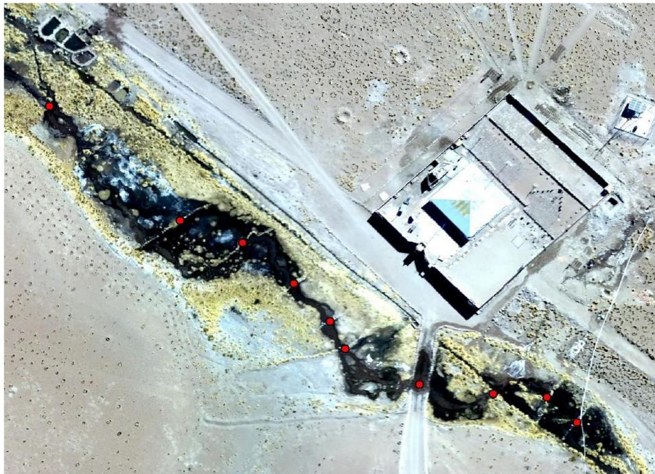
Figure 29 Example of obstructions to the flow. These obstructions should be dealt with individually in the hydraulic model as additional energy losses.
