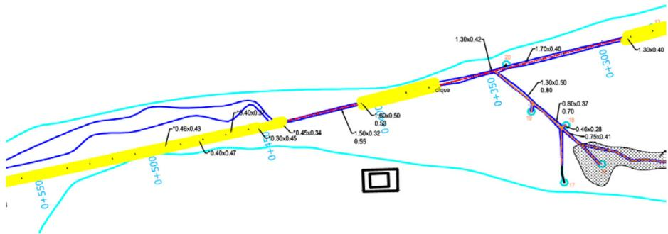
Figure 15 A close-up of the information of width and depth for canals in the Main Canal System from chainage 300 meters to chainage 600 meters (Southern wetland).
