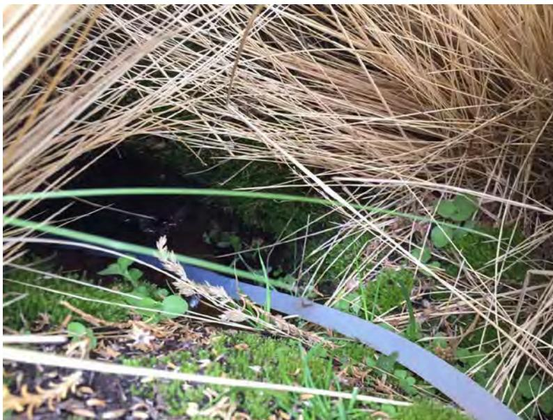
*Picture B1. Sampling of the spring SP-SI-5-17. The up gradient area was under vegetation, so the whole sample set was filtered using the peristaltic pump to avoid any type of contamination.*
