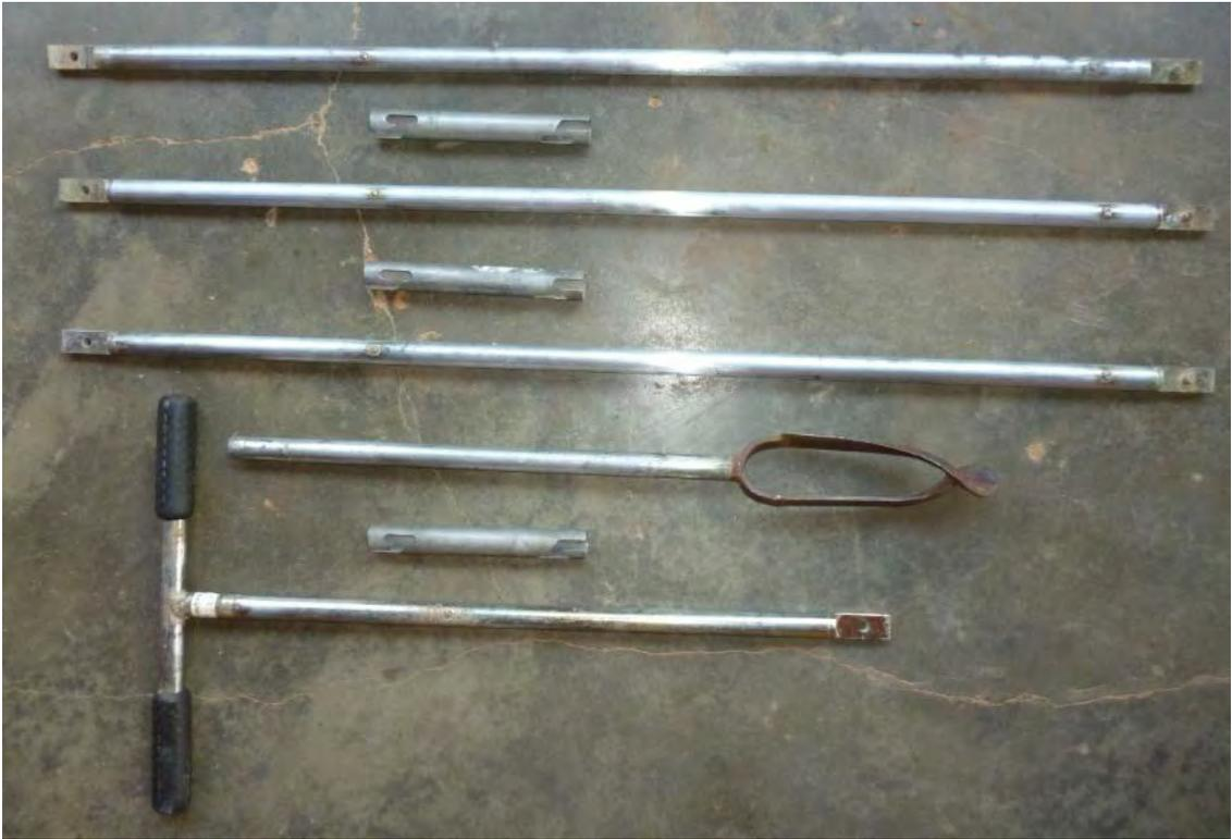
*Figure 4-10. Soil auger similar to that used at the Quebrada Negra wetland.*
