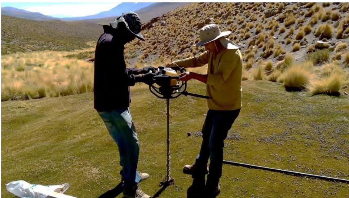
*Figure 4-21. Use of earth auger at study site.*
