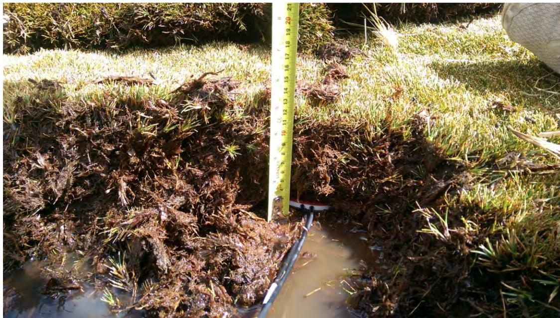
*Figure 4-5. Soil heat flux plate installation.*
