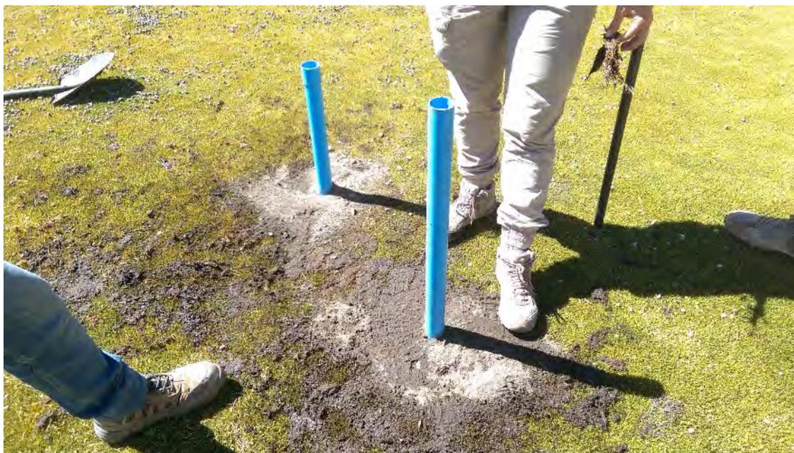
Figure 4-24. Pair of piezometers installed at test site 2.
