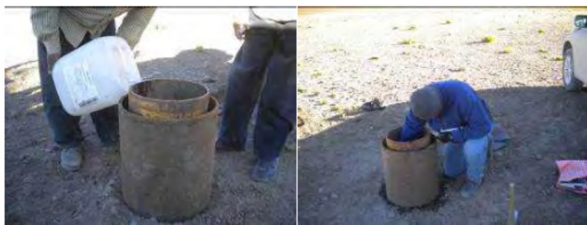
Figure N° 61. Infiltration test by means of the double ring in trial pit N° 7, which did not yield the expected results due to the excessive leakage of water through the lateral walls of the external ring to the required 3 cm [pipe] jacking.
