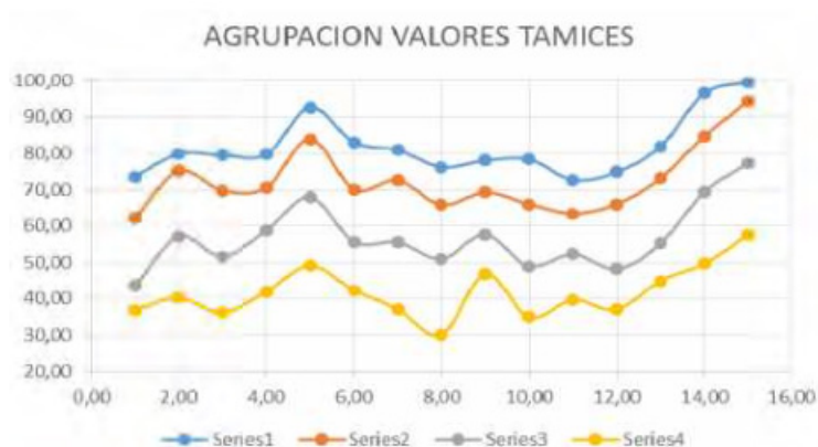
Chart N° 9. Curves interpolated with the data of the sieves N° 4, N° 10, N° 40 and N° 200 (Own Source).
