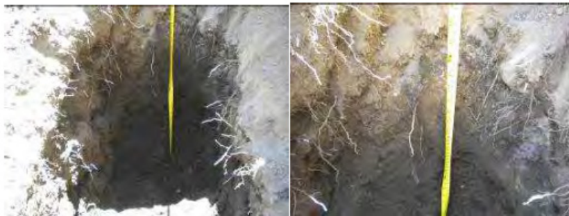
Figure N° 31: Presence of the rock mass; conclusion of the excavation works in the SLL-4 trial pit.
