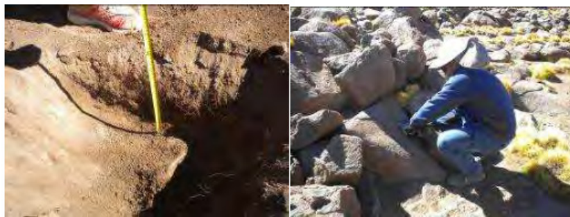
Figure N° 34: Presence of the rock mass; conclusion of the excavation works in the SLL-5 trial pit.
