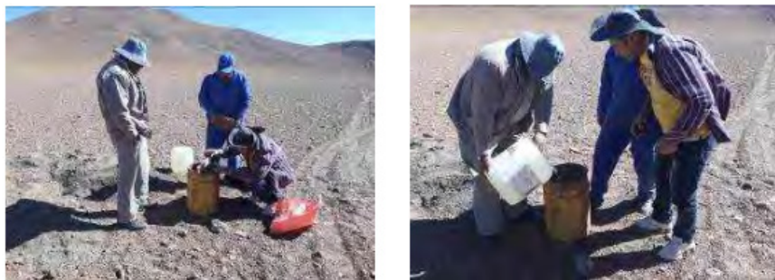
Figure N° 62. Infiltration test in SLL-8 trial pit.
