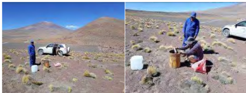
Figure N° 64. Infiltration test in the SLL-12 trial pit in sands with a silty matrix with a maximum thickness of 1.00 meters in depth, where there is the presence of rocky basement composed of ignimbrites and lavas (Sanguenza 2018).
