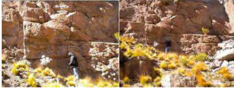
Figure N° 29: Measurement of joints in the rock mass.
