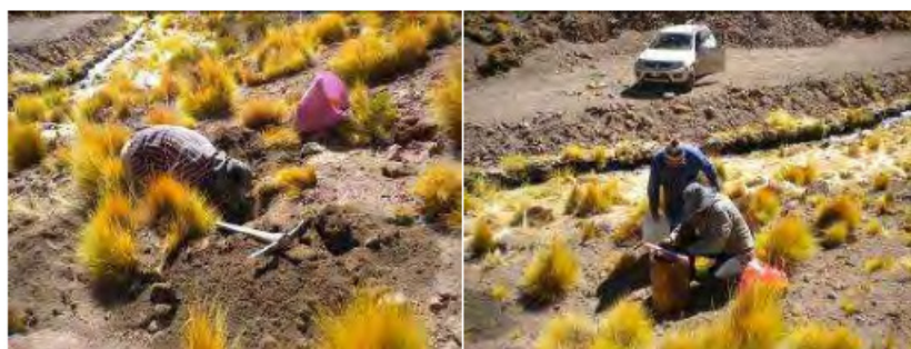
Figure N° 65. Excavation of the SLL-15 trial pit, carrying out the infiltration test using a ring in highly
