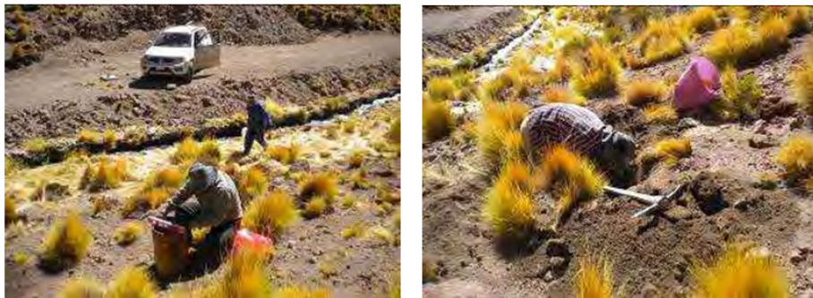
Figure No. 4. Trial pit excavation, SLL-15, on colluvial fan deposits composed of sands that contain clast fragments. One of the sections where infiltration tests were completed.
