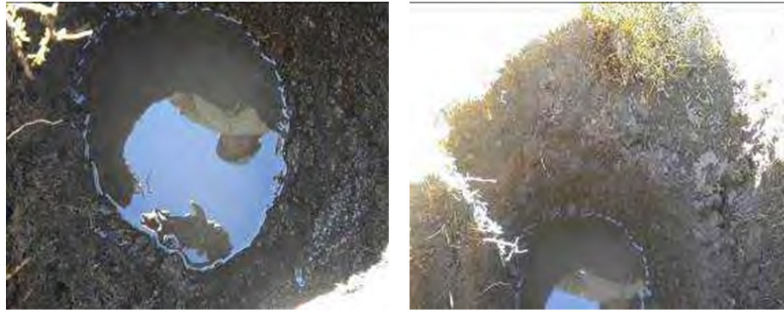
Figure No. 6. Infiltration test completed in the SLL-1 trial pit. It did not present a drop in the water level during the first fifteen minutes of the test.
