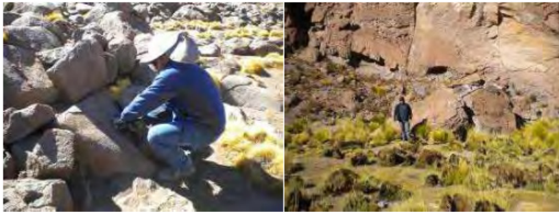
Figure N° 19. Measurements of planes of joints that present the igneous rocks through which the surface waters that infiltrate the granular materials flow.
