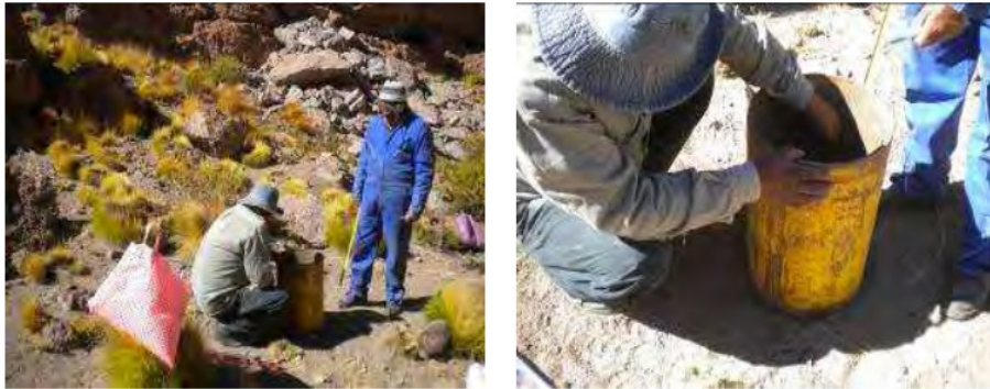
Figure No.7. Infiltration test completed in the SLL-4 trial pit, in silt-matrix sands, using a single ring due to the problems experimented when trying to set up the double ring infiltrometer
