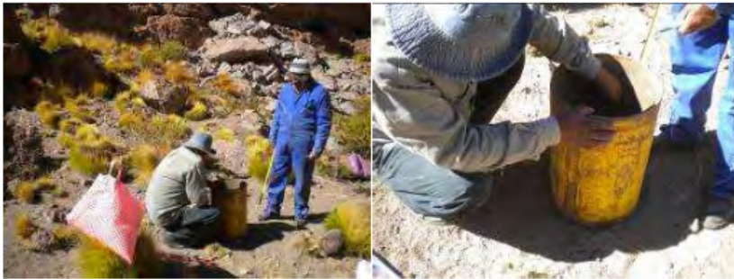
Figure N° 60. Infiltration test in the SLL-4 trial pit in silty matrix (SM) sands, using a single ring due to the problems presented when the double ring was armed.
