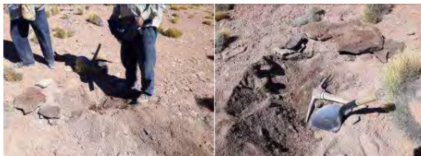
Figure N° 16. Presence of the almost surface rocky basement in the SLL-13 trial pit, where there is the presence of sandy materials with a silty matrix.
