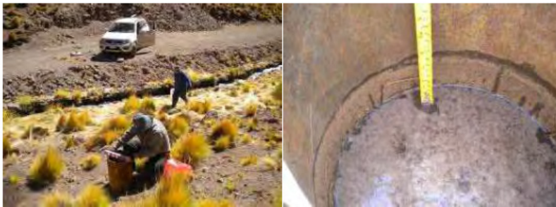
Figure N° 17: Infiltration velocity measurement in SLL-15 trial pit.
