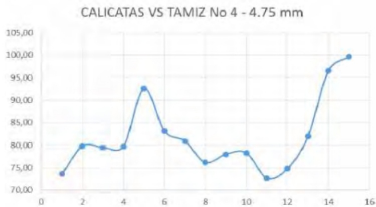
Chart N° 5. Representation of the percentages obtained in the fifteen soil samples through sieve N° 4 (Own Source).
