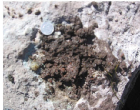
b) Sediments in the upper zone of the South Bofedal canal (Site 1, D_m = 0.3 cm)
