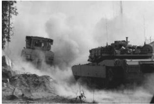
The CTS micro-combined arms team; D7 Armoured Bulldozer with an M1 Tank
